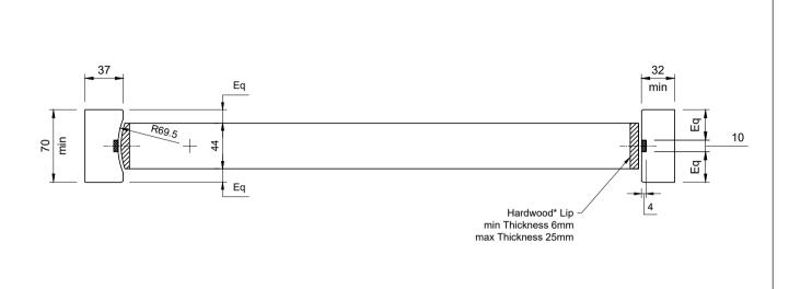
70 min Eq Eq 15 32 min Hardwood\* Lip min Thickness 6mm max Thickness 25mm Hardwood\* Lip min Thickness 6mm max Thickness 25mm max
